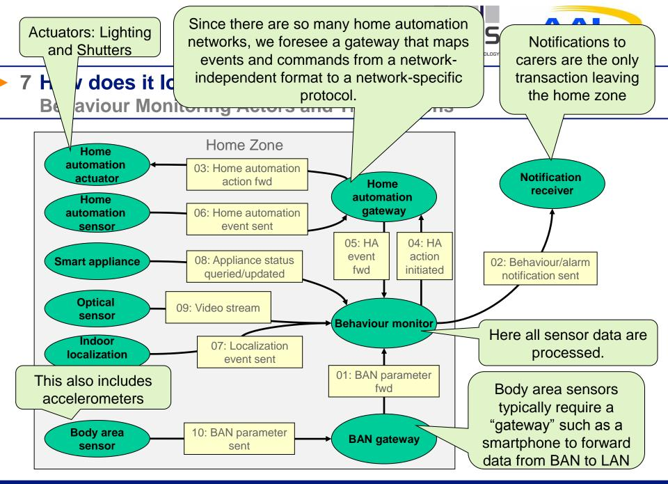
A home automation sensor generates a measurement and sends it using KNX (cabled) or ZigBee (wireless) to the home automation gateway
